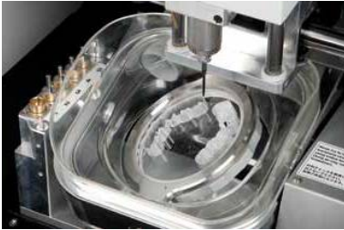
5-Axis machine 1 (Roland DWX-50, for dental applications).
